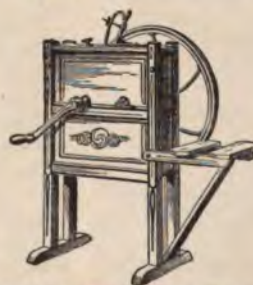
Fig. 91. One-hole corn-shellers. The larger one has a capacity of sixty to eighty bushels per hour; weight, 290 pounds.
